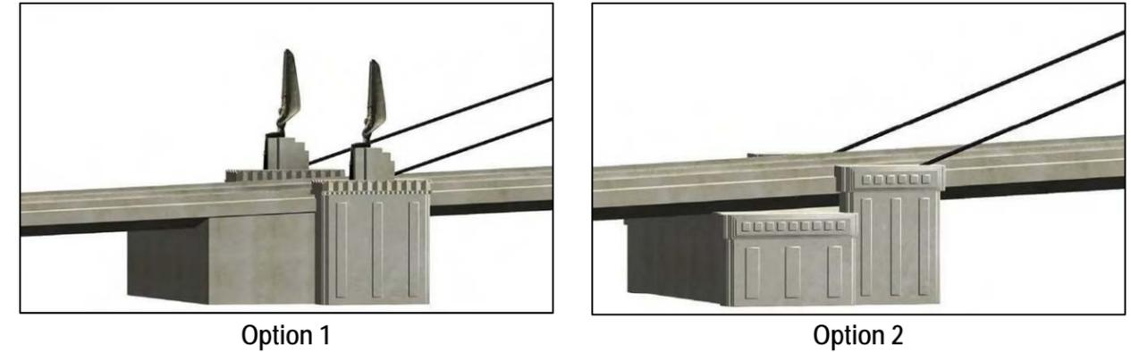
Figure 3.3-15 Suspension Bridge Anchorage Preferences
